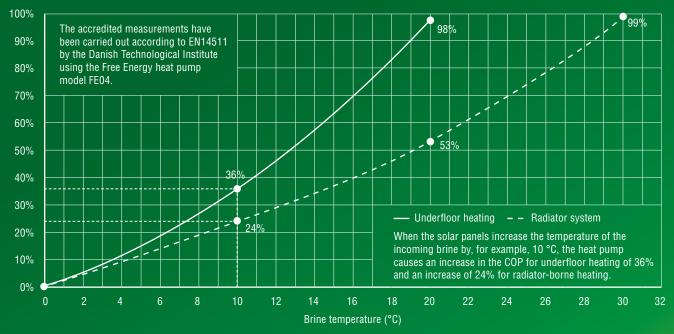
This halves the pay-back time for the solar panels in combination with HYSS, since solar heating is used both for hot tap water and to increase the efficiency of the heat pump.
