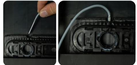
Figure 36 : Panel temperature probe
