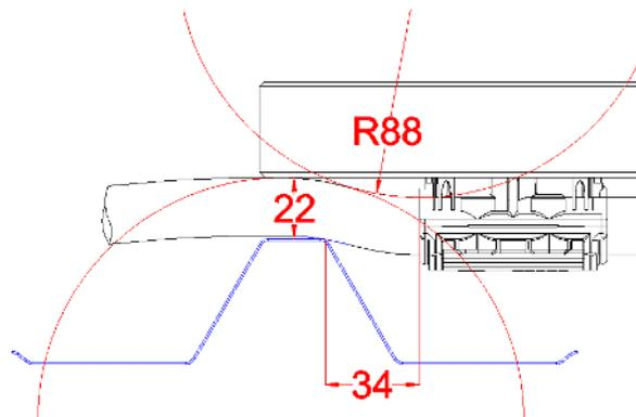
Figure 14 : DN15 hydraulic link routing through corrugation crest
