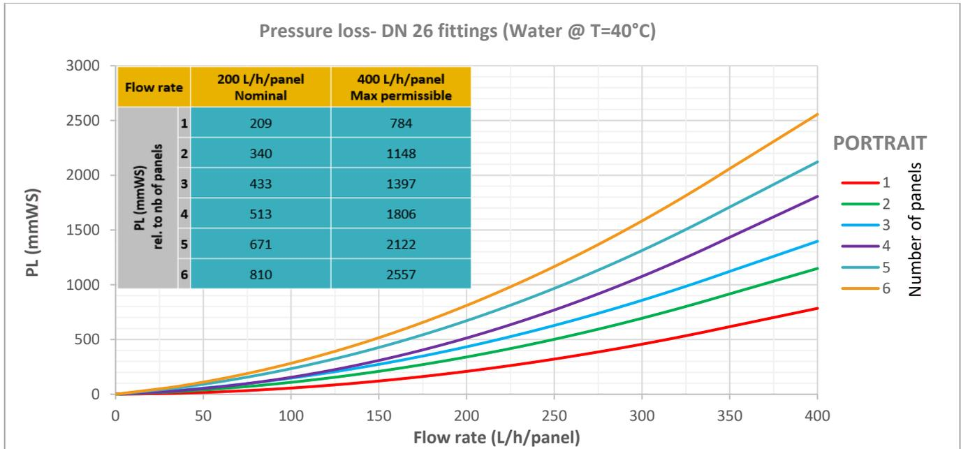
Figure 6 : Pressure loss curves for DUALSUN Spring XXXM – 60 – 3BBPN panels in portrait with DN26 fittings
