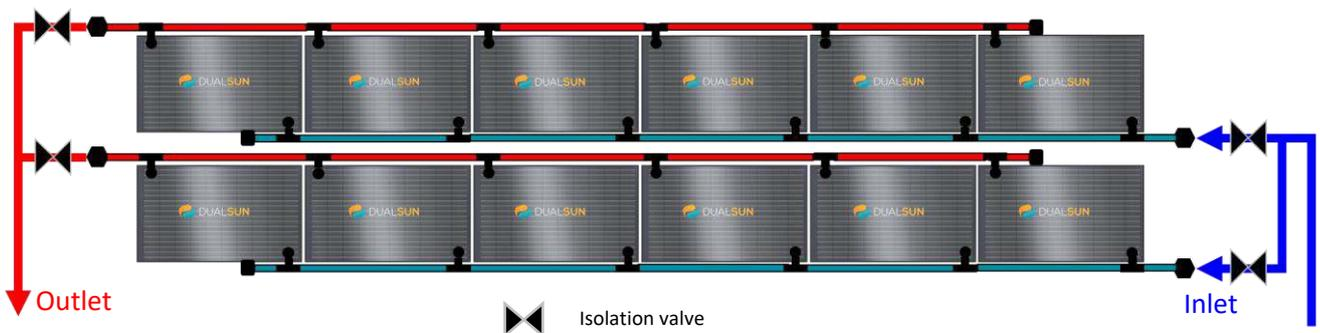
*Figure 27 : Hydraulic balancing – Pressurised system
