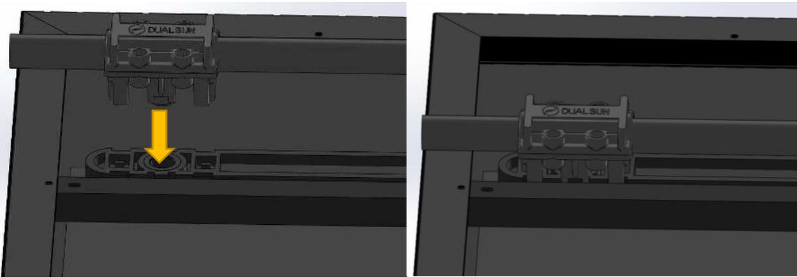
Figure 24 : Plugging of the DualQuickfit hydraulic fittings into the Spring Panel collector
