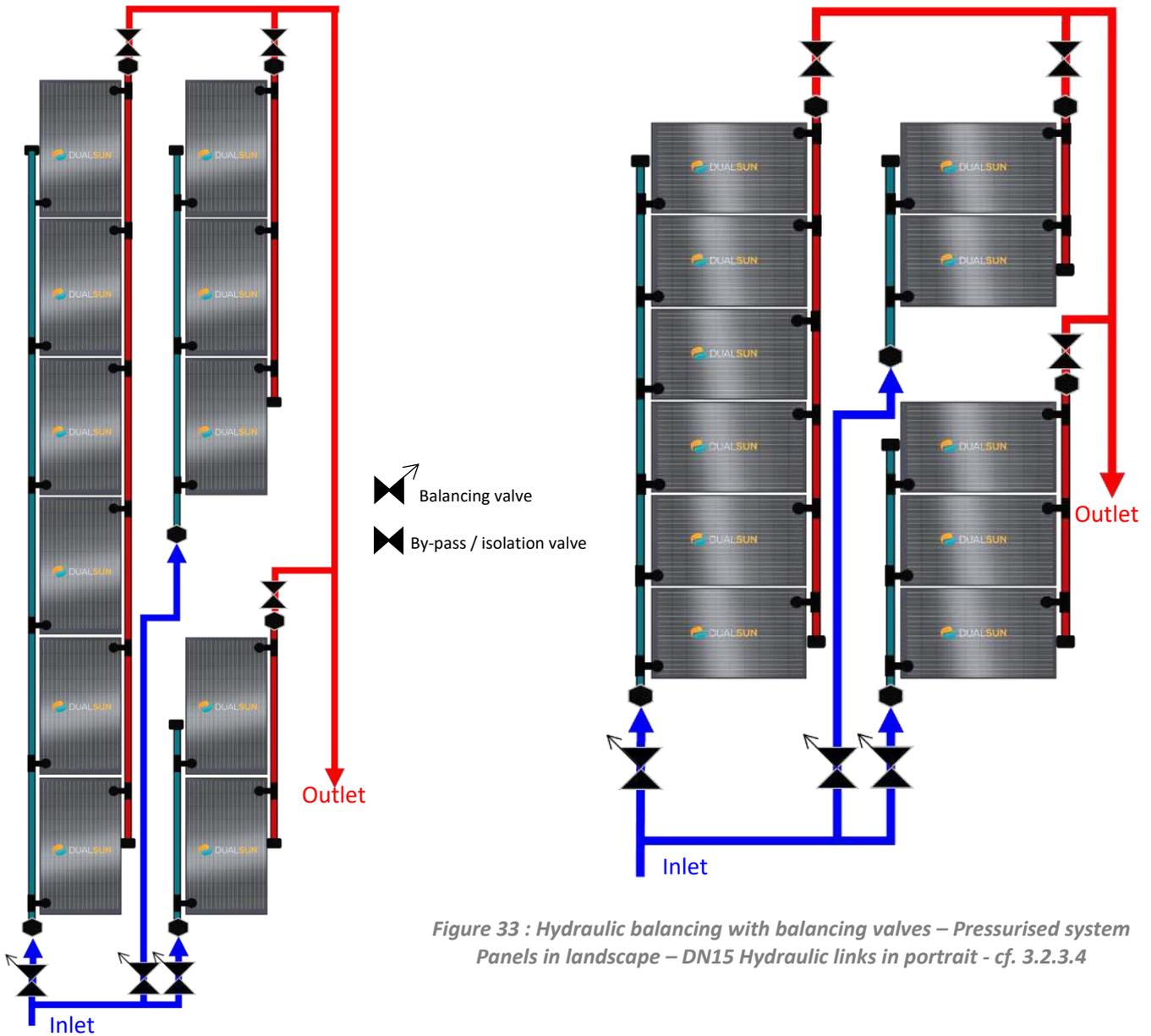
Figure 33 : Hydraulic balancing with balancing valves – Pressurised system
