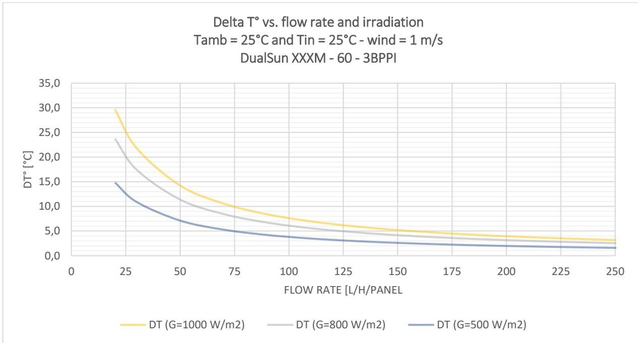
Figure 2 : Delta T = f (Q) curves for DUALSUN Spring XXXM – 60 – 3BPPI – insulated version
