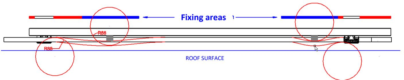
*Figure 19 : Rails avoidance in portrait with DN26 hydraulic links*
