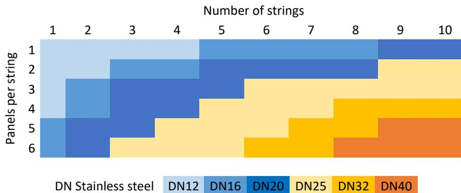
**b. Pressurised system –Thermal discharge –Nominal flow rate = 100 L/h/panel**
