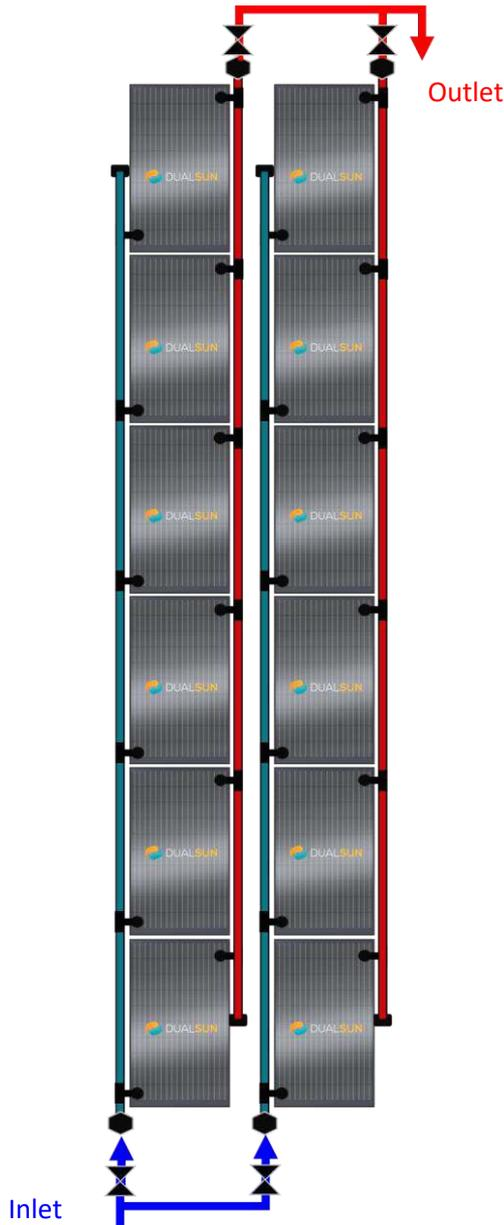
*Figure 28 : Hydraulic balancing – Pressurised system
