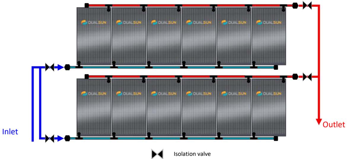
*Figure 26 : Hydraulic balancing – Pressurised system
