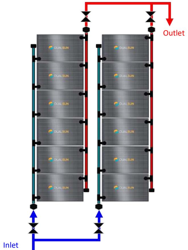
*Figure 29 : Hydraulic balancing – Pressurised system
