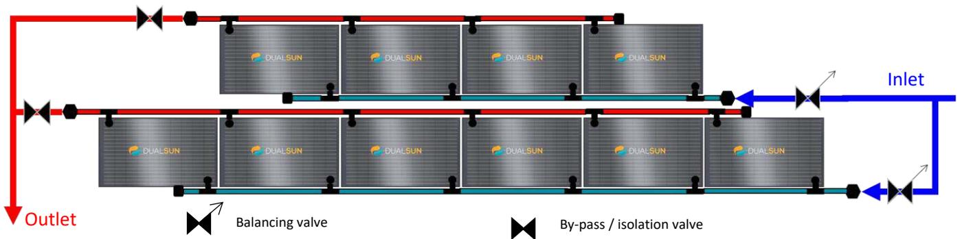
*Figure 31 : Hydraulic balancing with balancing valves – Pressurised system
