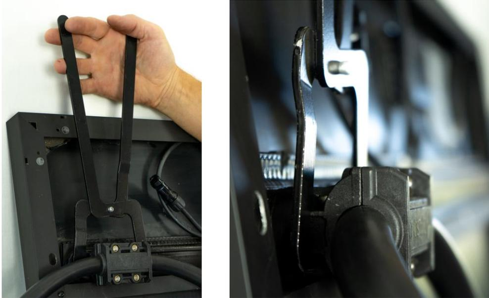
Figure 37 : Disassembly of DualQuickfit hydraulic fittings
