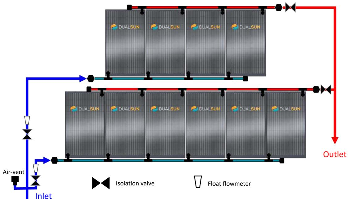
*Figure 35 : Hydraulic balancing – Direct pool heating system
