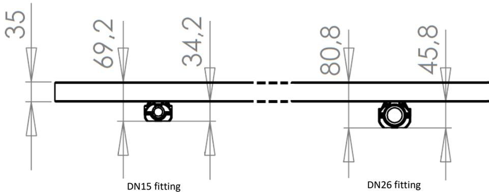
Figure 9 : Overall dimensions of hydraulic connections on the rear panel
