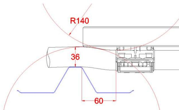
Figure 15 : DN26 hydraulic link routing through corrugation crest
