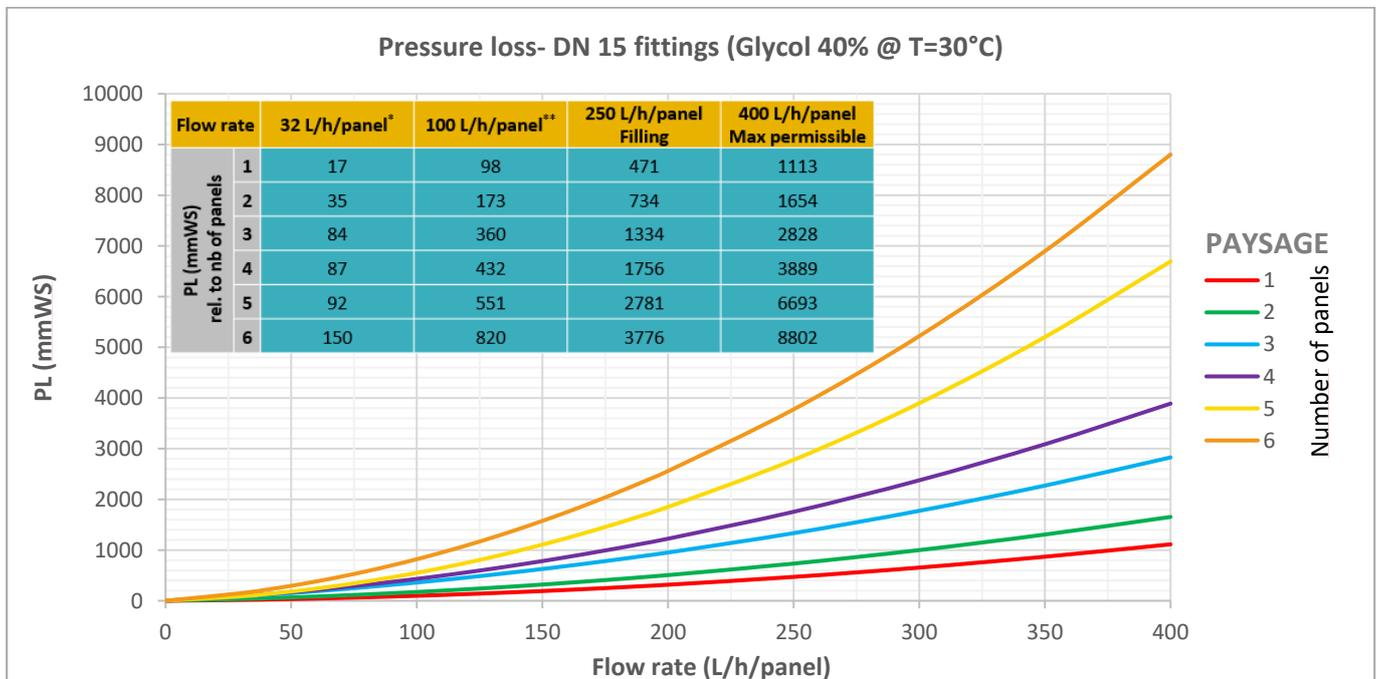
Figure 5 : Pressure loss curves for DUALSUN Spring XXXM – 60 – 3BBPI and 3BBPN panels in landscape with DN15 fittings
