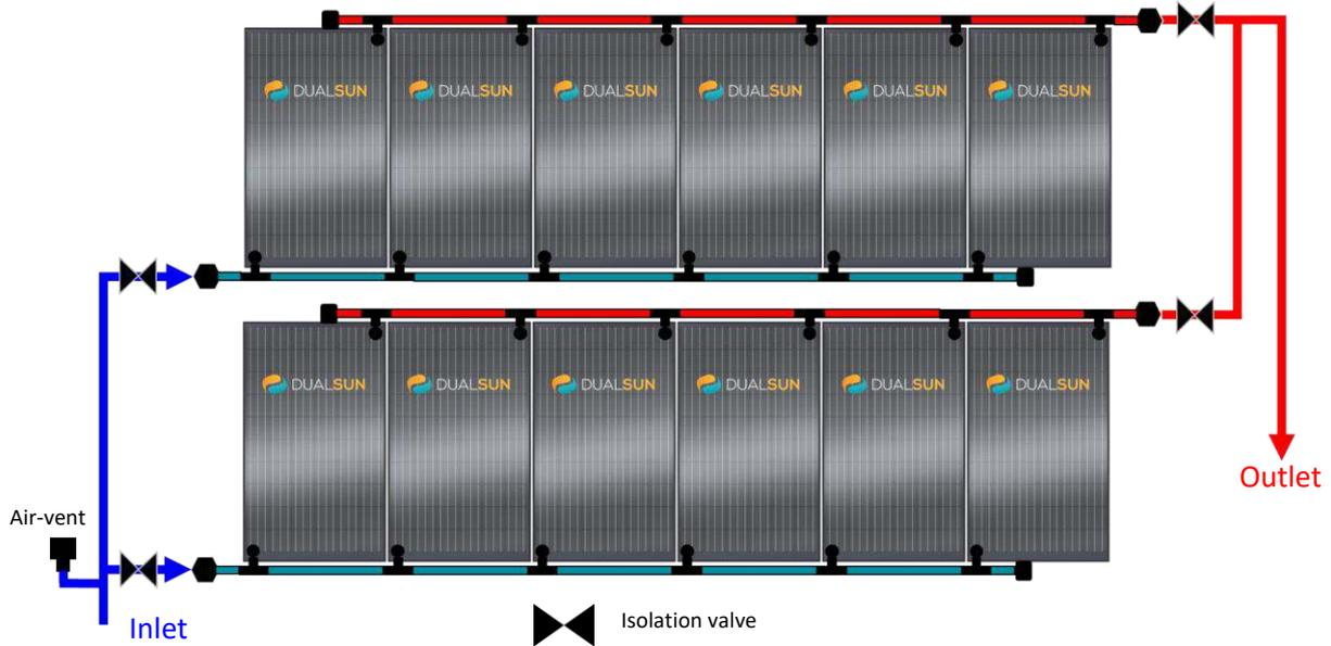
*Figure 34 : Hydraulic balancing – Direct pool heating system
