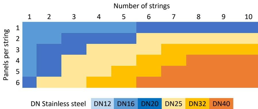
c. Direct pool heating system – Nominal flow rate = 200 L/h/panel
