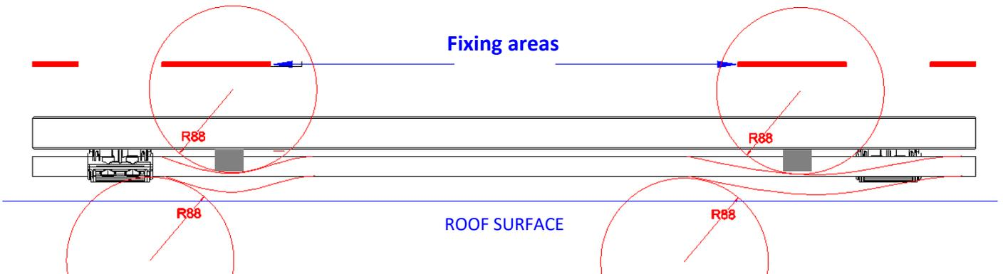
*Figure 18 : Rails avoidance in portrait with DN15 hydraulic links*
