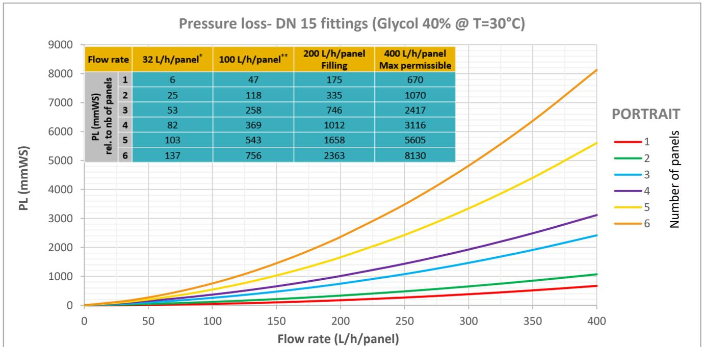
Figure 4 : Pressure loss curves for DUALSUN Spring XXXM – 60 – 3BBPI and 3BBPN panels in portrait with DN15 fittings
