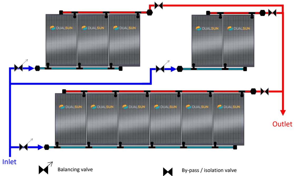
*Figure 30 : Hydraulic balancing with balancing valves – Pressurised system
