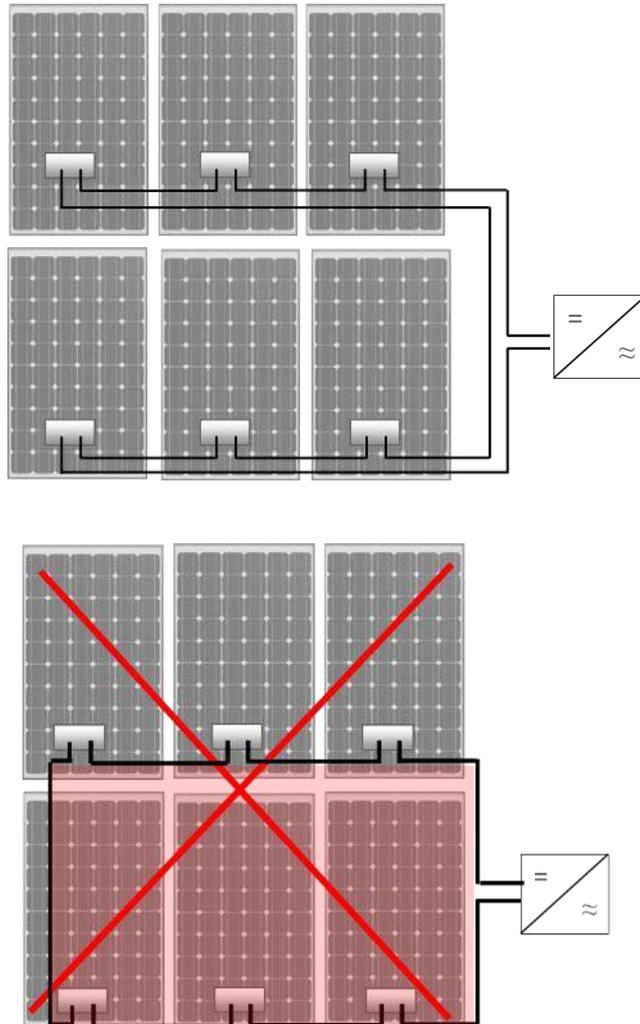
Figure 22 : Simplified diagrams showing two examples of good and poor grounding of a PV field
