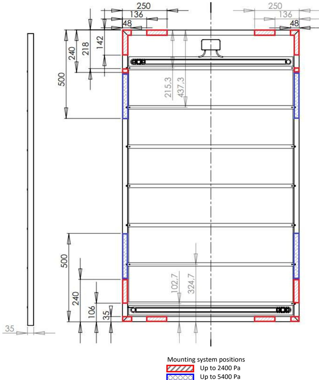
Figure 8 : Possible positions of the clamps to fasten DualSun XXXM-60-3BBP panels
