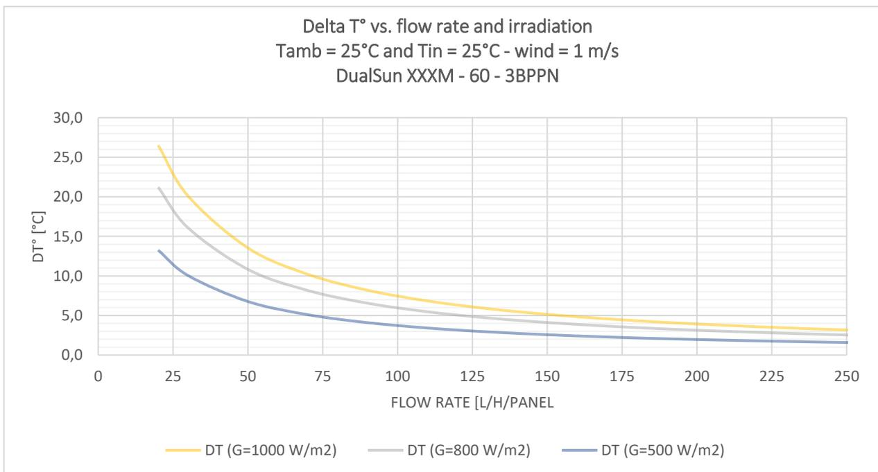
Figure 3 : Delta T = f (Q) curves for DUALSUN Spring XXXM – 60 – 3BBPN – non-insulated version
